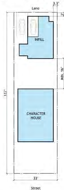
Figure 6 – Parking configuration for infill on 33 ft. lot
